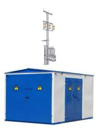
settlements, agricultural consumers, garden cooperatives, oil and gas fields, industrial facilities located in regions with a temperate climate. Equipped with additional equipment for street lighting control. The power of the power transformer is from 25 kVA to 63 kVA. This type of substation is not used in places of high vibration load and at explosive objects [3].
