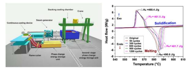
Fig. 2 – Device structure & Thermal cycle simulation results
