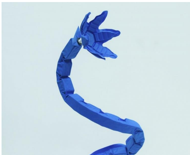
Figure 2. Fluid-driven origami-inspired artificial muscle
