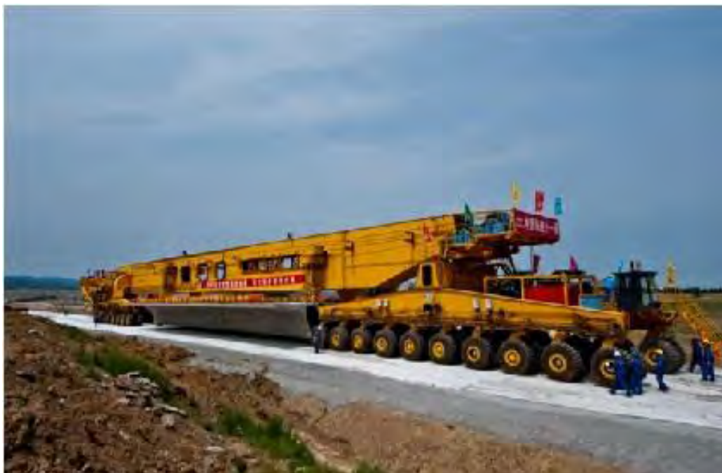
Рисунок 1 – SLJ900/32 Segmental Bridge Launching Machine.
