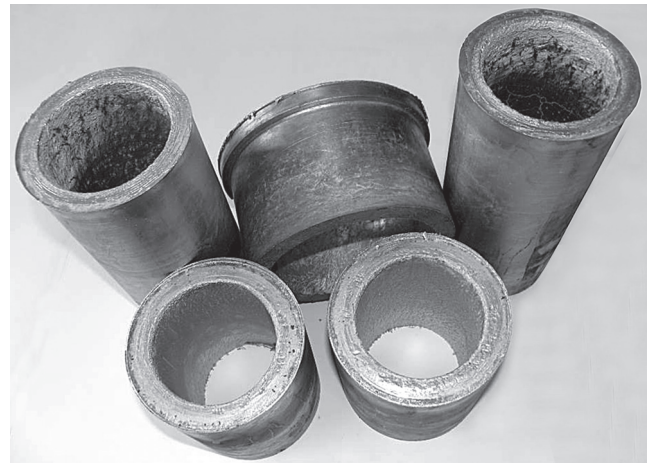
Fig. 4. Hollow castings of antifrictional silumin
