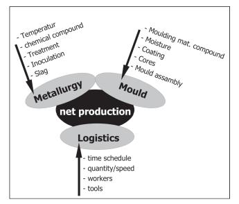
Fig. 1. Possibilities for influencing the casting result
