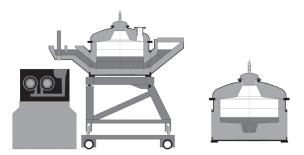
Fig. 5. The Unheated Pouromat® pouring system
