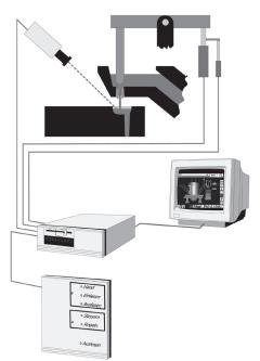
Fig. 7. Diagram of a Laser-Controlled Pouring Stream
