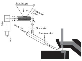
Fig. 8. Pouring Stream Inoculation Monitoring System
