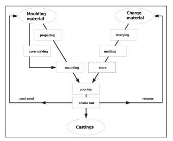
Fig. 2: Simplified Diagram: Principal Material Flow Circuit to pour the material into molds in conformity with defined requirements.
