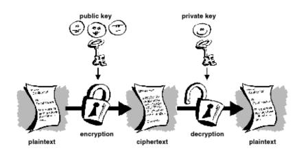
Figure 41 – Demonstration of encryption-decryption process using private and public keys
