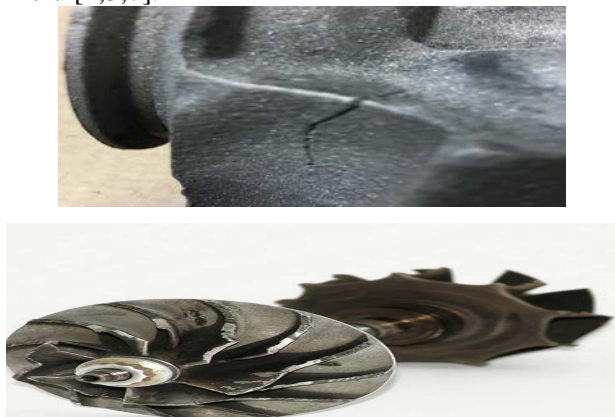
Fig. 2. Fracture of the outer part of the housing
