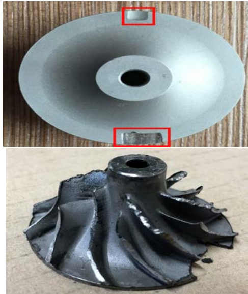
Fig.10. Mass reduction points on the compression wheel
