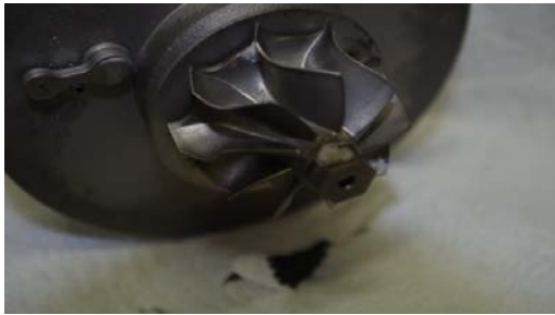
Fig.14. Mass on the turbine wheel after compression test Fig.15. Ripped wheel masssss
