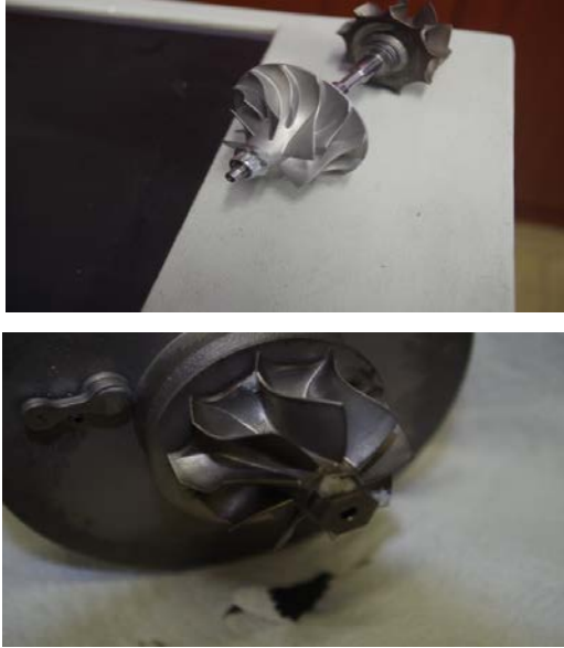
Fig.14. Mass on the turbine wheel after compression test Fig.15. Ripped wheel masssss
