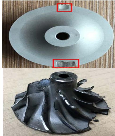
Fig.10. Mass reduction points on the compression wheel
