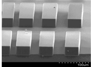
Fig. 2 - SEM photo of 230 µm thick microstructures based on the SU-8 2150 photoresist
