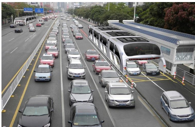
The Straddle bus station platform
