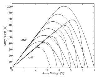
Fig. 1. Array power versus its voltage for the temperature of (from right to left) 273,300, 325,350,375, and 400 K. Solid lines for AMO (air mass) condition, and dash lines for AM1 condition
