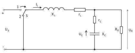
Fig. 5. Lumped parameter model of the buck converter
