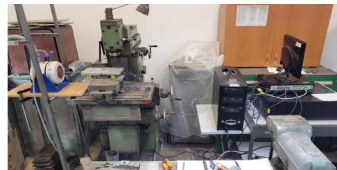
Figure 1 – Modal test of dynamometer using shaker input signal in longitudinal direction
