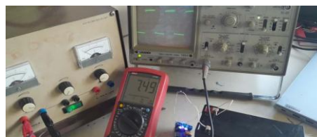
Figure 4 – Output waveform at 25 kHz and 50 % duty cycle with stabilized output voltage of 7.49 V
