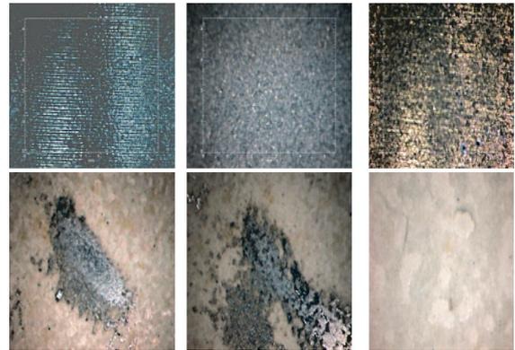
Figure 2. Roll surface images of different coatings after testing
