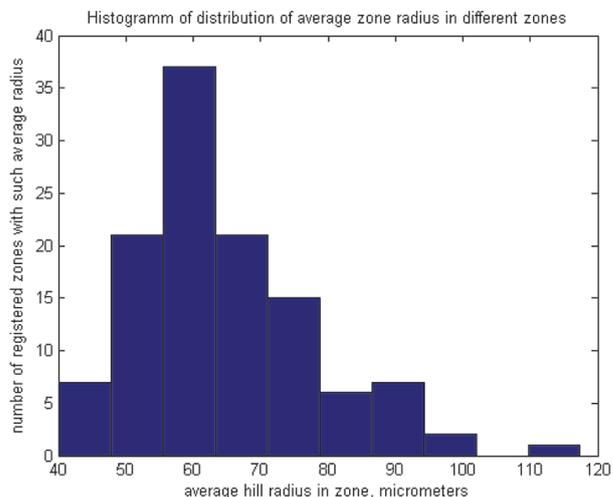
Figure 8. Distribution of average pickup radius in different zones of roll
