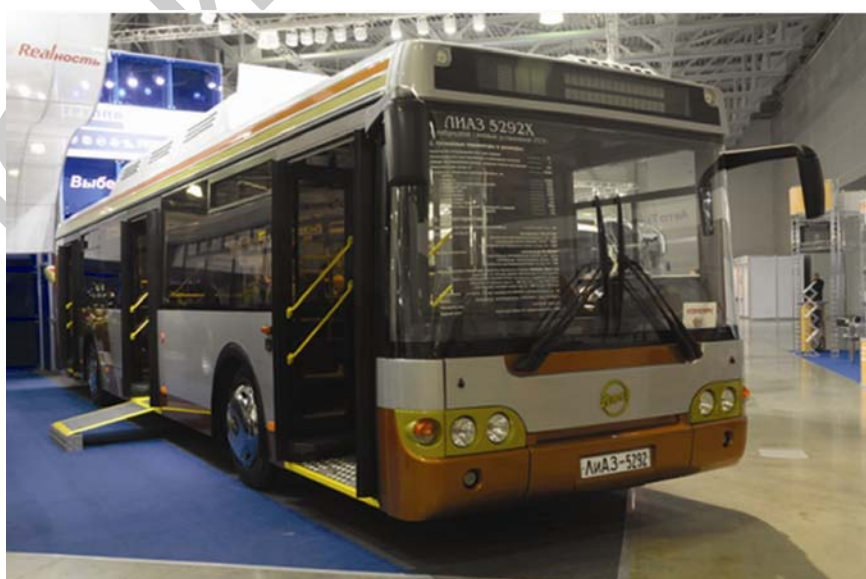
Figure 1: LIAZ 5292XX bus (prototype) with a hybrid drive train at International Automobile Forum (the KROKUS-EXPO epicenter, Moscow, September 9-12 th , 2008).
