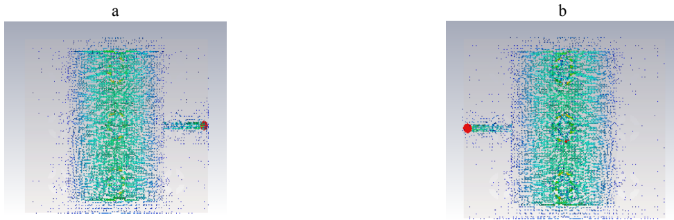
Fig. 9. Distribution of surface current in the proposed antenna (a) front (b) back
