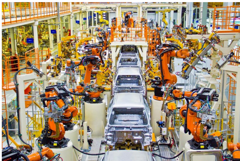
Fig. 1. – KUKA robots on the main welding line
