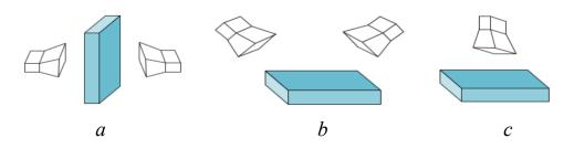
Figure 1 – System diagram of sample measured by free space method: a – transmission method; b – double antenna reflection method; c – single antenna reflection method
