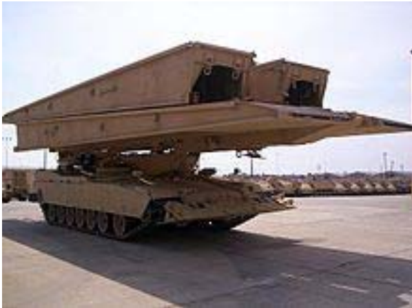
Fig. 17.2. U.S. Army M104 Wolverine Heavy Assault Bridge
