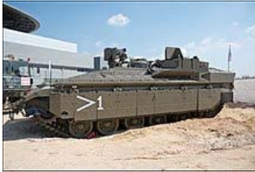
Fig. 16.1. IDF Namer CEV (is used both to carry section of sappers and to operate combat engineering devices)
