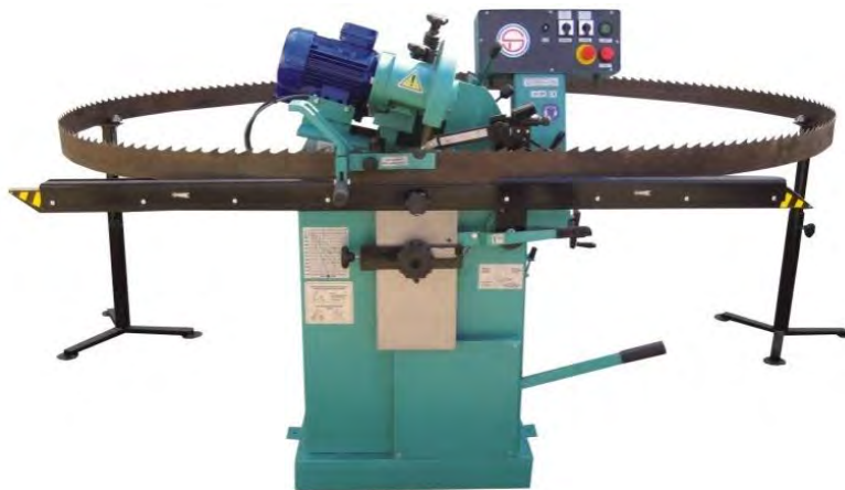
Fig. 1. Universal sharpening machine OS-2M
