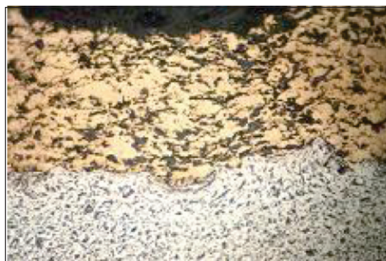
Fig 17 – The Ni coating on steel
