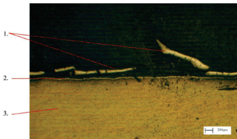
Fig. 6 – The structure of deposited coating with low current density: 1 – hard-chrome coating, 2 – bond coat (nickel), 3 – base material (aluminium)
