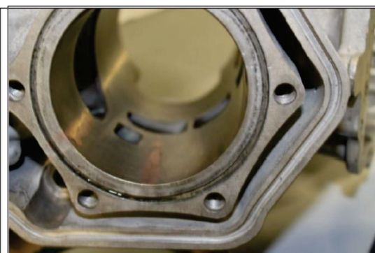
Fig. 19 – The renovated scratch in in engine block
