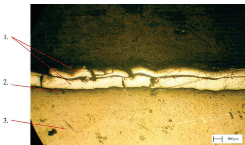
Fig. 7 – The damaged structure of hard-chrome coating: 1 – hard-chrome coating, 2 – bond coat (nickel), 3 – base material (aluminium)
