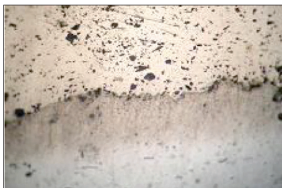
Fig 12. The Ni Zn coating on aluminium
