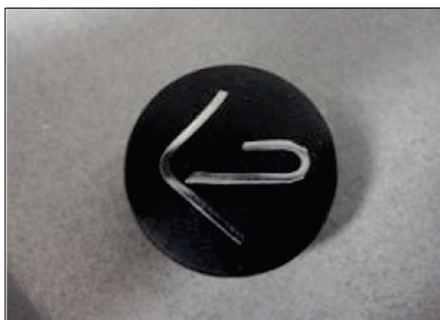
Fig. 8 – The the coating bond strength tested samples
