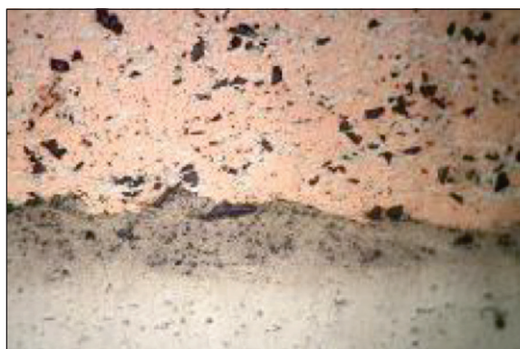
Fig 14 The CuZn coating on aluminium alloy
