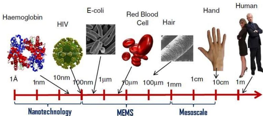
Fig. 1 - Dimensional scale of MEMS and Nanotechnology
