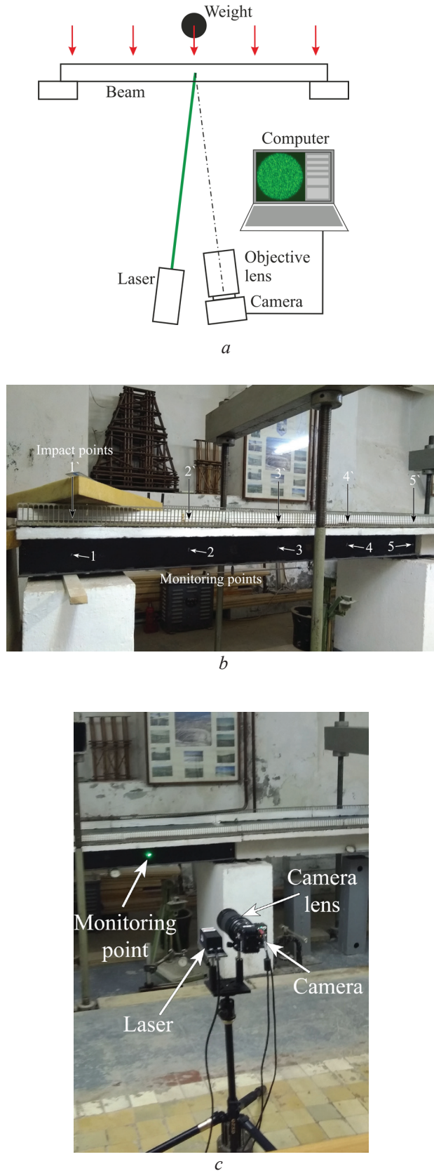
Figure 2 – Scheme of the experiment with dynamic loading by a free fall of steel disk (a); photographs of the laboratory bridge model (b, c)
