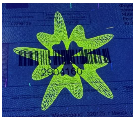
Figure 4 – Invisible protective image, fluorescent fibers under ultraviolet light
