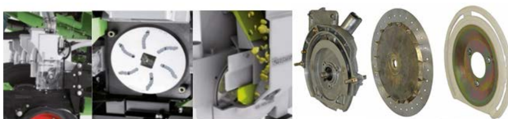
Figure 1 – Structural diagram of the Wintersteiger seeder part and MONOSEM seed metering device
