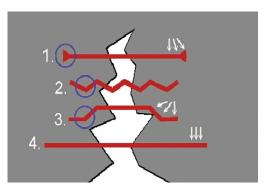
Fig. 4. Influence of different types of wire fiber on crack resistance: *I* – cone anchors fiber, *2* – wavy fiber, *3* – crooked ends fiber, *4* – straight fiber (blue circles – mechanisms of fiber anchoring, white arrows- adhesion surfaces)
