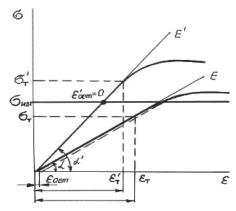
Fig. 5. Residual deformation of wire with different elastic modulus:  $\sigma_T$ ,  $\sigma_T$ , – yield points of wires with different elastic modulus;  $\sigma_{\text{M3T}}$  – tension at unbending of anchor fiber end under tensile load;  $\varepsilon_T$ ,  $\varepsilon_T$  – elongation at flexible area of wire with different elastic modulus;  $\varepsilon_{\text{oct}}$  – residual deformation after load in plastic area; E, E' – elastic moduluses of different wire materials (E' > E)
