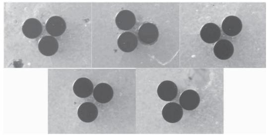
Fig. 6. Geometrical location of wires in steel cord 3x0,30 HT FRP
