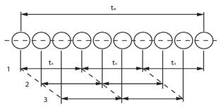
For better penetration of a rubber compound projections of deformed adjacent wires on to longitudinal axis of steel cord are shifted as regards to each other as shown in Fig. 4.
