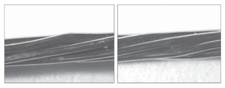
Fig. 7. Steel cord 0,40 + 6x0,38 HT FRP appearance. ×16
