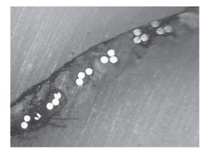
Fig. 12. Cross-section of a rubber-steel cord strip
