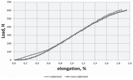
Fig. 9. Elongation diagram of 3x0,30 HT FRP rubberized and non-rubberized
