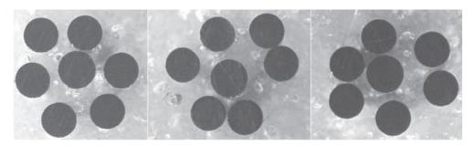
Fig. 8. Transverse arrangement of wires in steel cord 0,40 + 6x0,38 HT FRP
