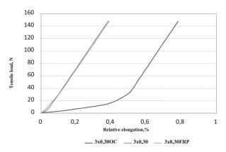
Fig. 11. Comparison of elongation diagrams of steel cord 3x0,30 with various deformation of separate filaments
