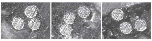
Fig. 13. Segments of a rubber-steel cord strip: geometrical arrangement of wires after calendaring
