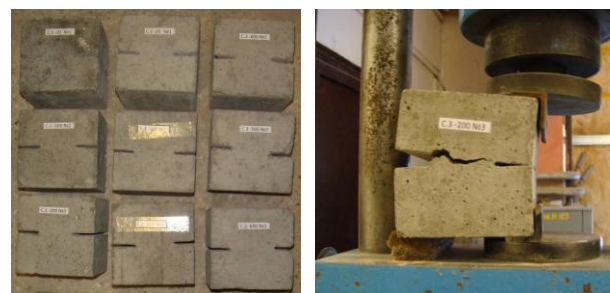
Fig. 2b. Specimens before and after K_{IC} tests
