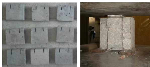
Fig. 3b. Specimens before and after K_{IC} tests
