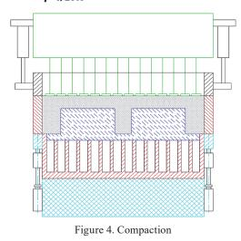
After detailed consulting, Kutes Metal decided to use the SEI-ATSU.*plus* process. The 'plus' variant includes an auto-level frame as supplementary equipment, improving compaction of the pattern sides. This substantially increases mold strength, particularly at the mold's edges.
