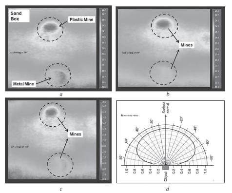
Fig. 6. The mines locations; images taken at (a)  $90^\circ$ , (b)  $60^\circ$  and (c)  $-60^\circ$ ; (d) emissivity values at different angles
