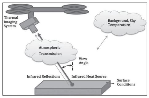
Fig. 2. Thermal Imaging System
