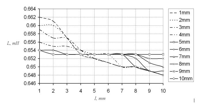
Figure 3 – Measurement results of particle concentration in MRF on different levels of fluid Numbers indicate values of ultrasonic horn immersion depth
