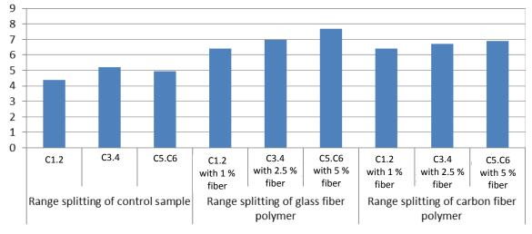
*Fig. 3.* Comparison between control samples cubes against fiber glass reinforced polymer and carbon fiber reinforced polymer in flexural strength
